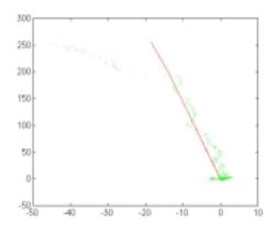
Figure 12 Comparison of DGPS and Kinematic Solution
