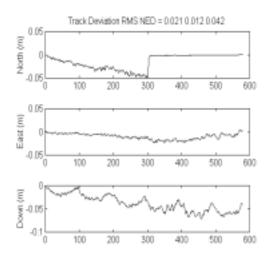
Figure 11 Kinematic GPS Test Data
