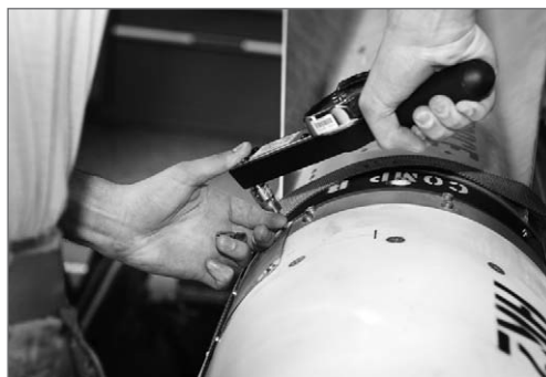
A member of the 86 th Munitions Squadron removes the guidance control section of an AGM-65 Maverick missile system for upgrades at Ramstein AB, Germany. By July 2011, more than 2,000 AGM-65 Maverick H and K models will have been updated.
