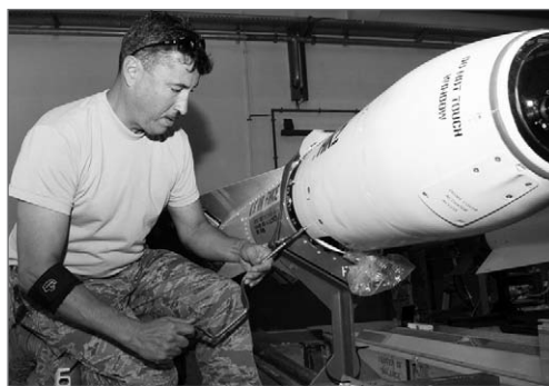
USAF Master Sgt. Eugene Rinaldi removes the guidance control section of an AGM-65 Maverick missile system for upgrades at Ramstein AB, Germany.
