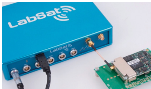
▲ FIGURE 11 LabSat GNSS simulator.
