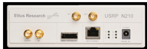
▲ FIGURE 2 Universal Software Radio Peripheral.
