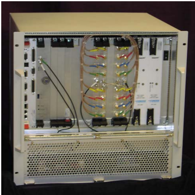
Figure 2 16-Element L1 Only Rack-Mounted SSGR
