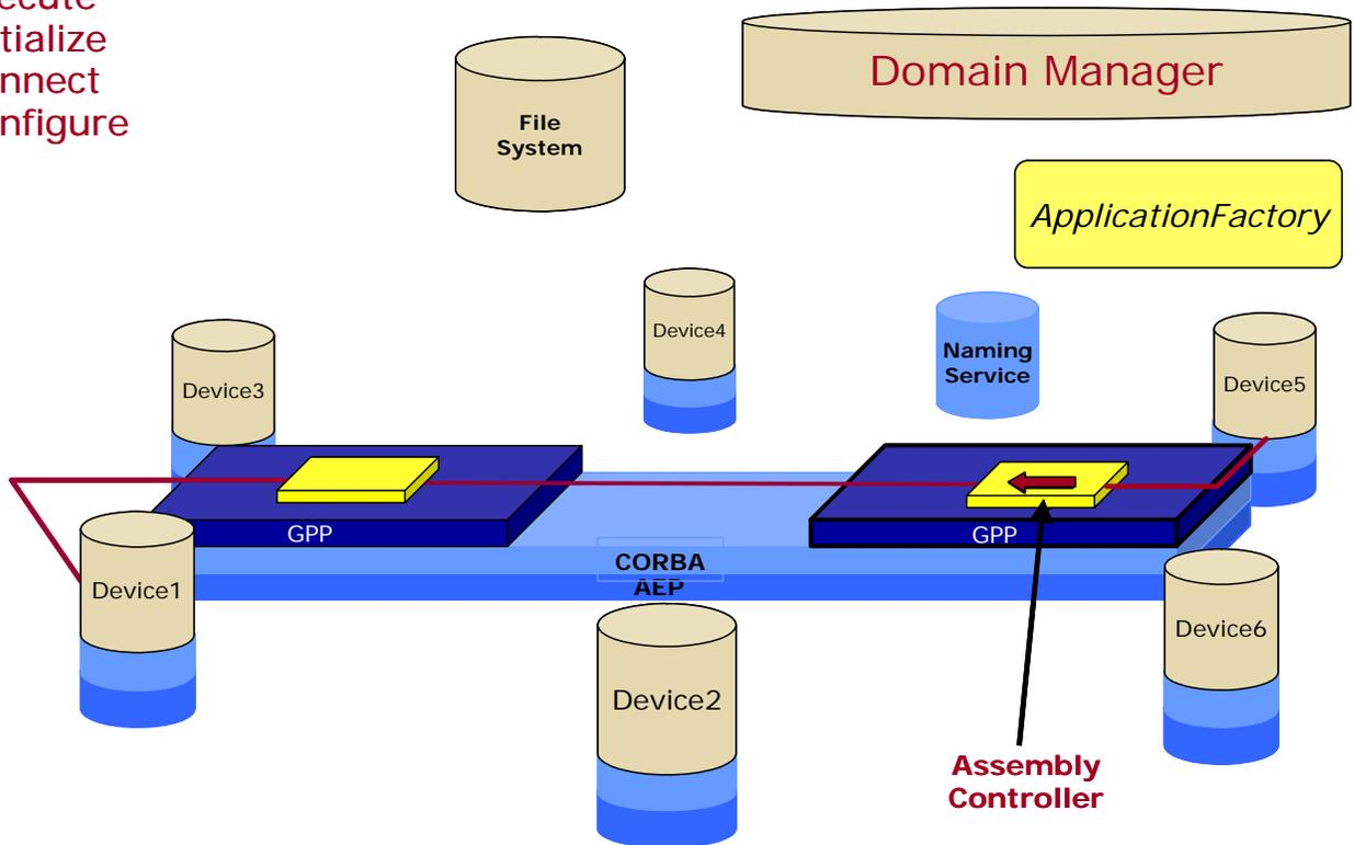
Figure 7 Waveform Instantiation and Configuration<sup>[5]</sup>
