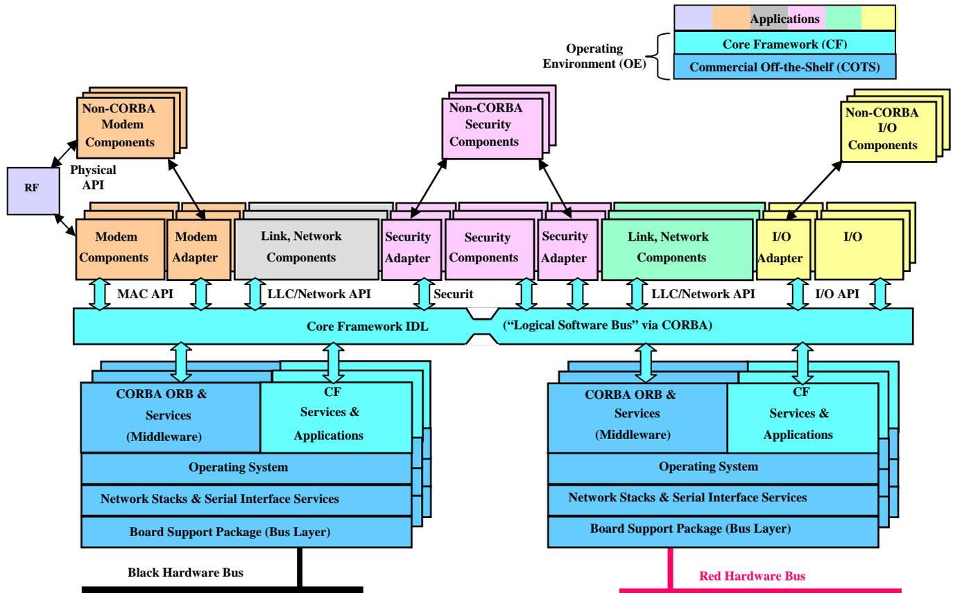
Figure 15: Software Communications Architecture and Operating Environment [7]
