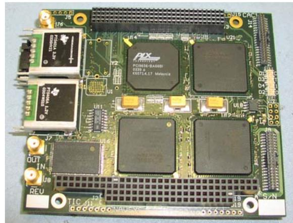
**Figure 13 PC/104 CAC FPGA Board**
