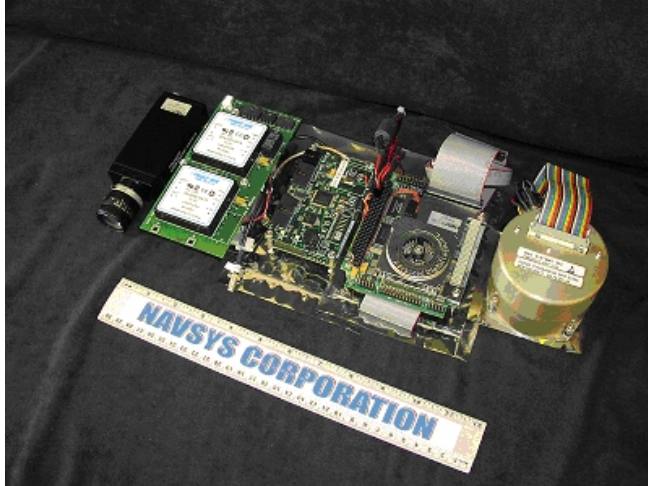
Figure 5 GI-Eye UAV Payload Components
