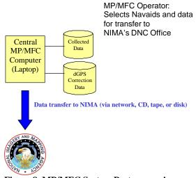
Figure 8 MP/MFC System Post-processing Architecture
