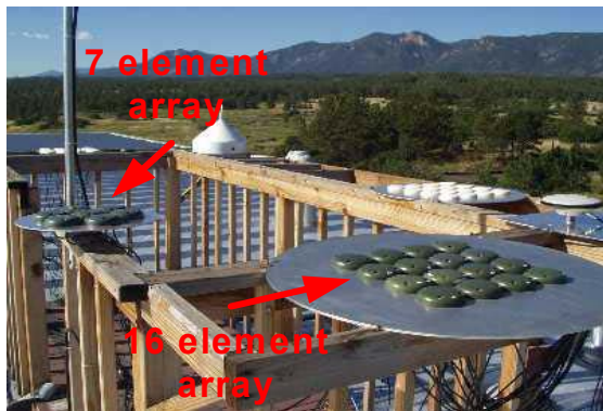
Figure 11 Two HAGR Arrays, Located on Roof
