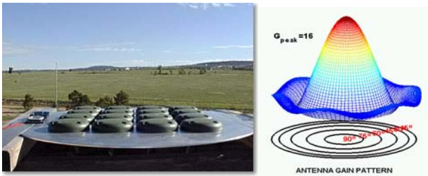
Figure 6 16 Element Array and gain pattern
