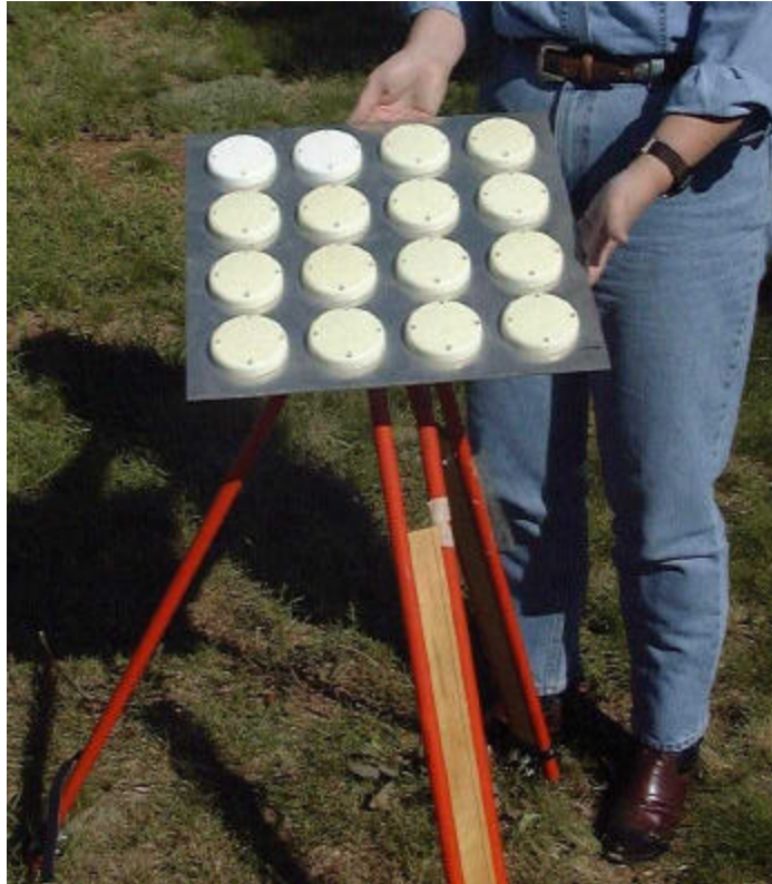
Figure 14 HAGR 16-element antenna array
