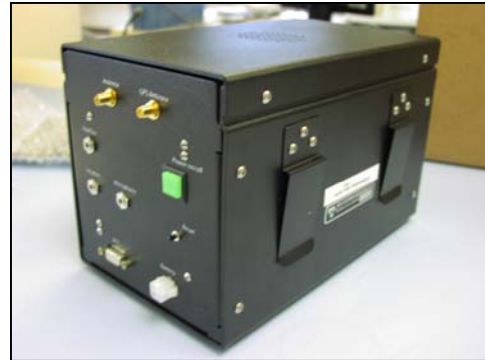
Receiver of the First Responder Communicator Tracking System
