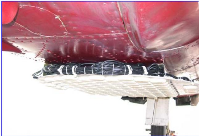
**96 Element Antenna Mounted on Aircraft**
