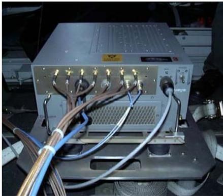
NAVSYS' High-gain Advanced GPS Receiver (HAGR) uses a digital beam steering antenna array to provide gain in the direction of up to twelve GPS satellites simultaneously on both the L1 and the L2 frequencies. This approach has the following advantages for precision GPS applications.
