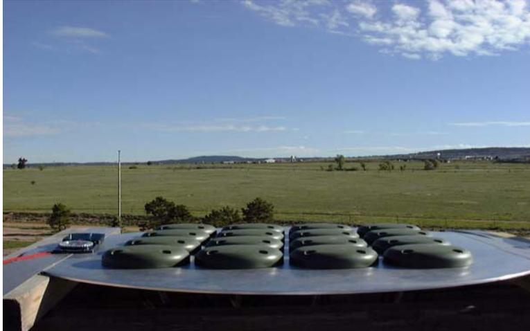
**Figure 6 Sixteen Element Antenna Array**
