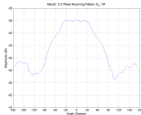
Figure 12 The x-z plane receiving pattern with E_\theta incident waves for AeroAntenna Technology’s AT575-97B-SMAF-000-00-00-NM GPS antenna
