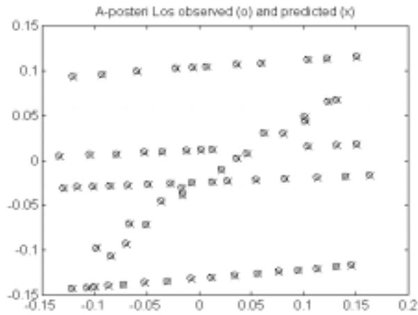
**Figure 5 Post Calibration Pixel Coordinate Errors (~0.3 mrad RMS)**
