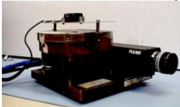
**Figure 2 GPS/Inertial/Video Sensor Assembly**
