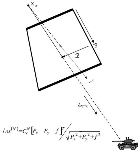
Figure 4 GI-View Target Location
