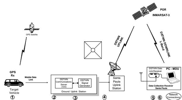
**Figure 9 DSTWN Test Architecture with Data Collection Points**
