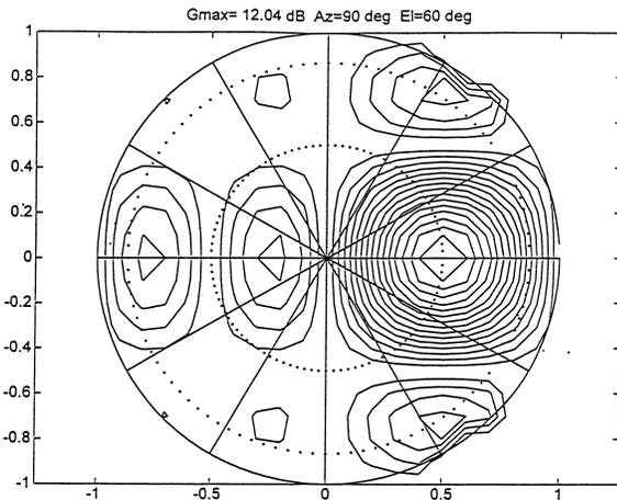
Figure 4 Single Satellite 16-element Digital Array Beam Pattern
