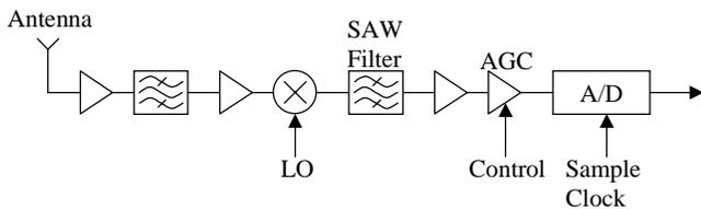
**Figure 3 Basic Front End Architecture**
