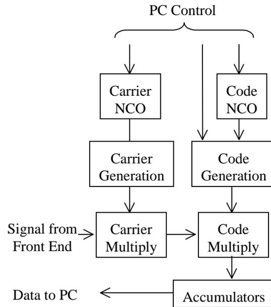
**Figure 5 Correlator Accelerator Card Functions**
