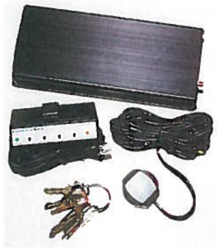
The in-vehicle unit's button-box driver interface can be attached to the driver's sun visor or kept in the glove compartment.
