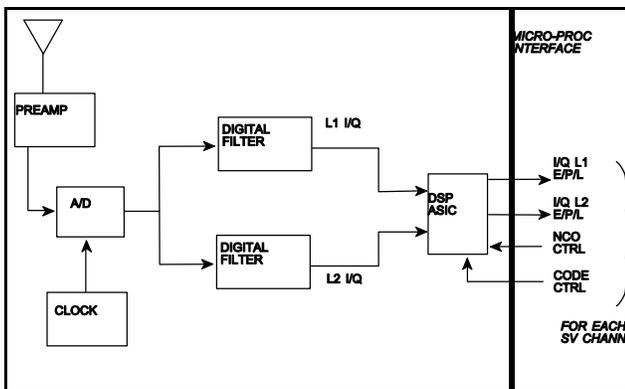
Figure 3 Advanced GPS Receiver (AGR)
