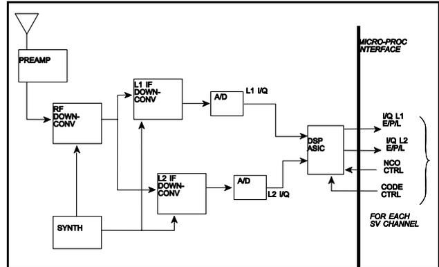
**Figure 2** Conventional Digital Receiver Architecture
