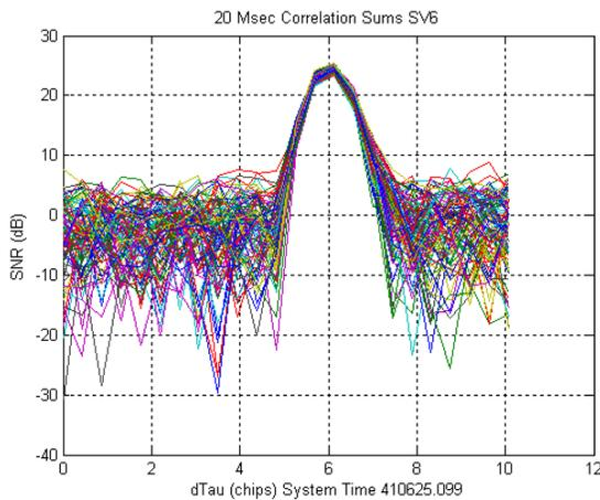
**Figure 7 20 msec Accumulation Results (SNR = 25 dB)**
