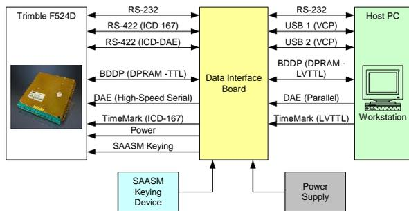
Figure 5 SAASM Interfaces for TIDGET Processing
