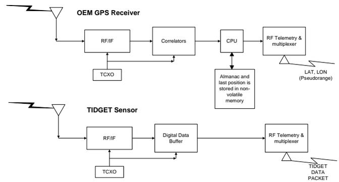
**Figure 1 TIDGET Sensor**
