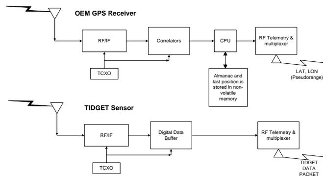
Figure 1-1 TIDGET Sensor
