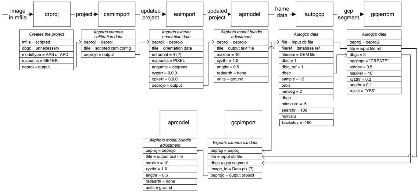
**Figure 6 Image bundle adjustment data flow**
