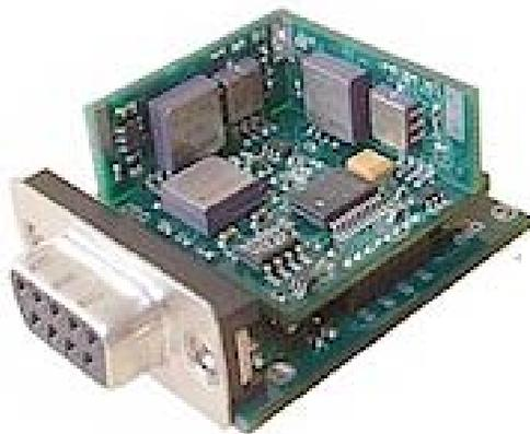
**Figure 5 Cloud Cap Crista IMU**
