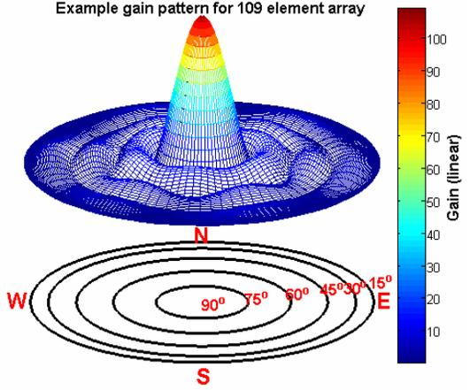
Figure 8 Beam Pattern of 109-Element Array
