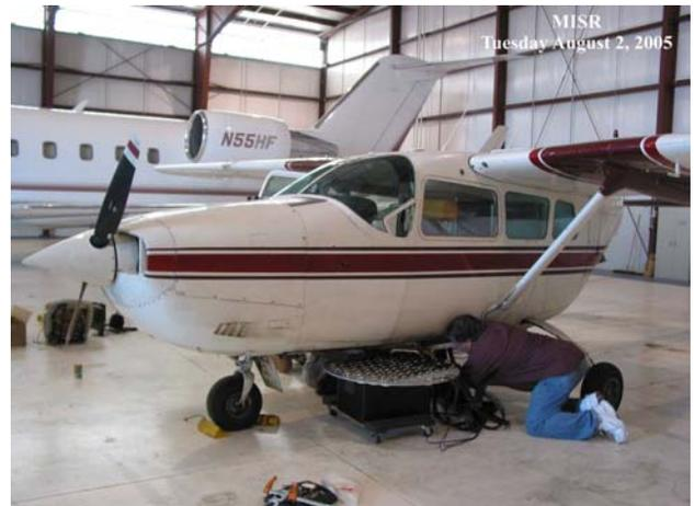
**Figure 4 96-Element Antenna Array Installation**
