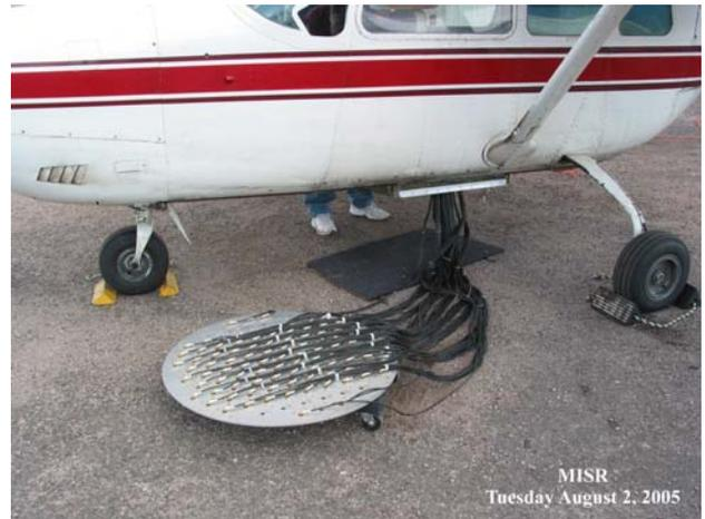
**Figure 3 96-Element Antenna Array before Installation**
