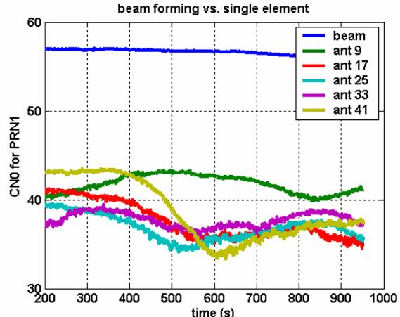
Figure 9 Beam forming Gain
