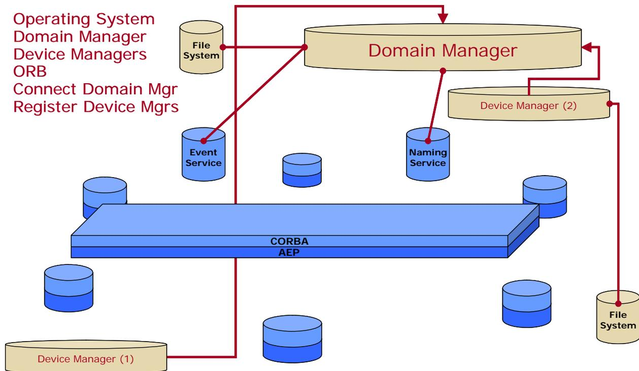
Figure 4 SCA System Start Up<sup>[5]</sup>
