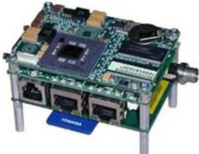
Figure 14 Ultra Miniature Computer (UMC)
