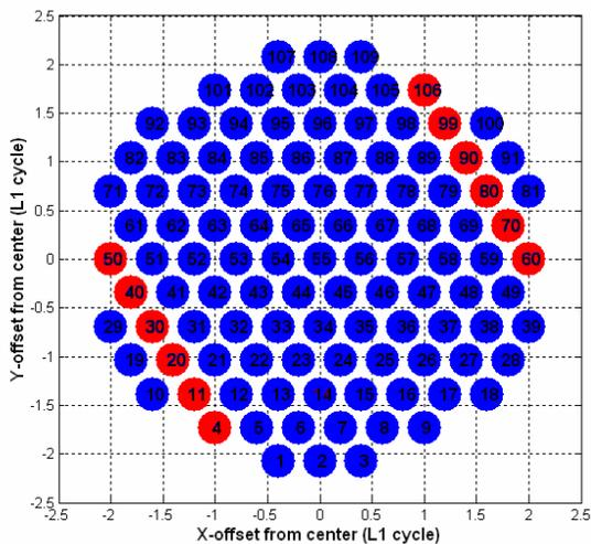
Figure 7 96-Element Phased Array
