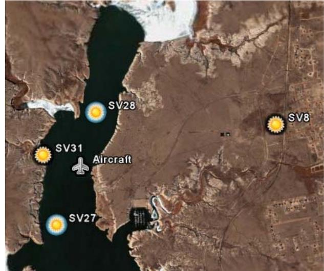
Figure 14 Aircraft and Specular Points over Land and Water
