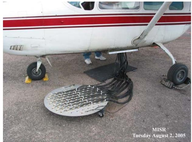
**Figure 3 96 Element Antenna Array before Installation**
