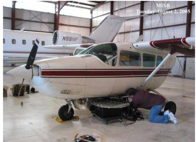
**Figure 4 96 Element Antenna Array Installation**
