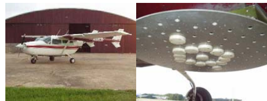
Figure 12 Cessna Test Aircraft and Antenna Array Mounted underneath
