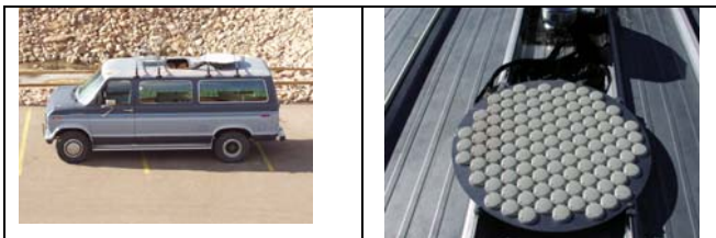
Figure 19 109 element array installed for van testing
