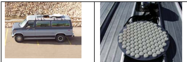
Figure 19 109 element array installed for van testing
