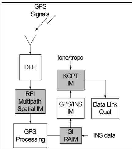
Figure 2 Integrity Monitoring Concept<sup>2</sup>
