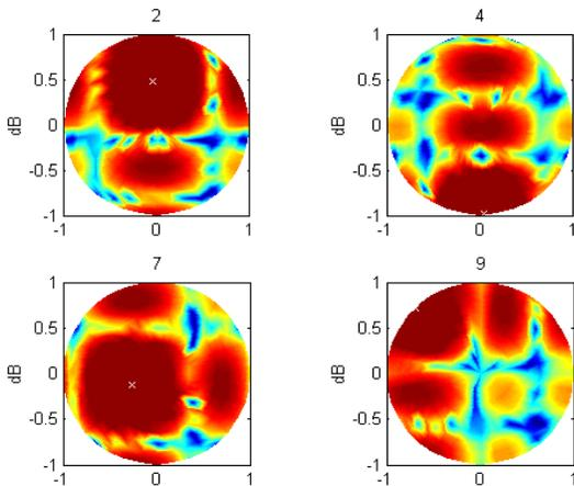
**Figure 7 L2 Beam Steering Antenna Patterns**
