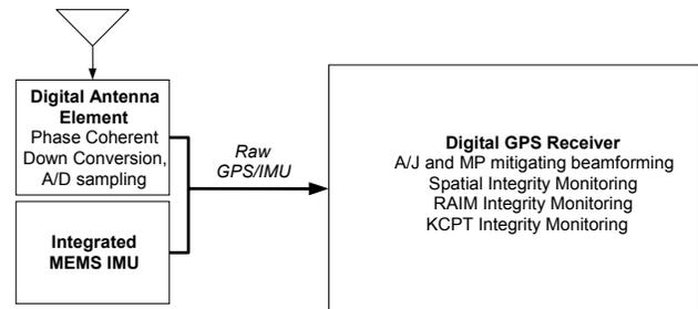
Figure 4 NAVSYS Digital Antenna Element and receiver
