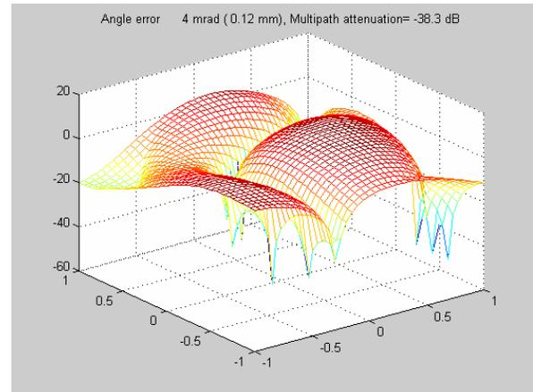
**Figure 8 Antenna Pattern with Multipath Mitigating Beam Forming**
