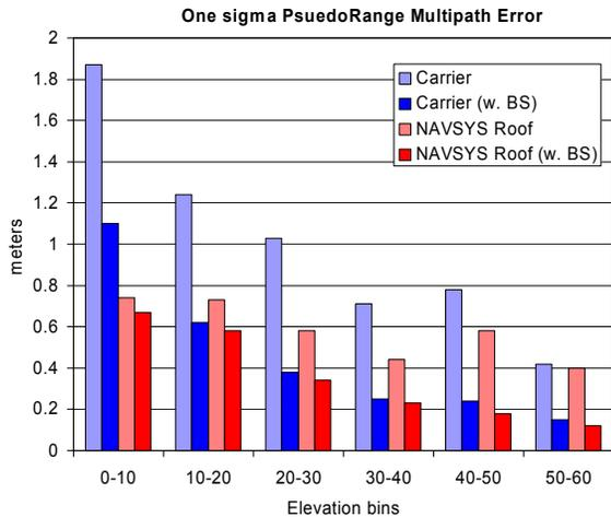
**Figure 19 Pseudorange MP Error as a Function of Elevation**
