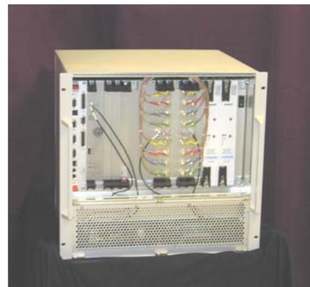
**Figure 9 PCI Form Factor HAGR receiver**
