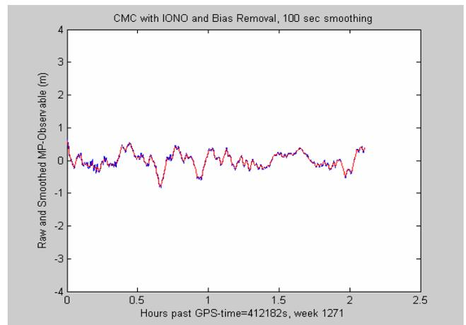
**Figure 17 CMC with Ionosphere Error Removed**
