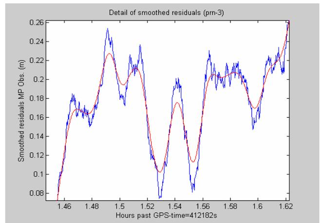
**Figure 18 CMC with Fit to Smooth Receiver Noise**
