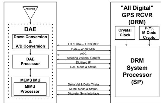
Figure 3 Current Generation DOD Digital Antenna Electronics
