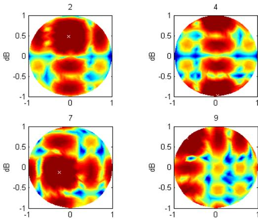
**Figure 6 L1 Beam Steering Antenna Patterns**
