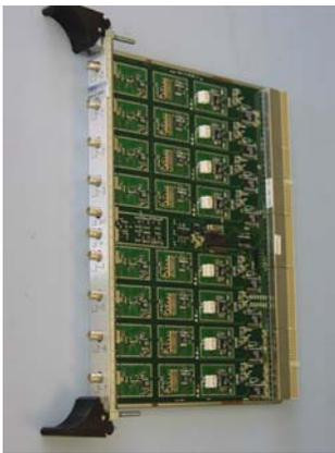
**Figure 10 Digital Antenna Element card**
