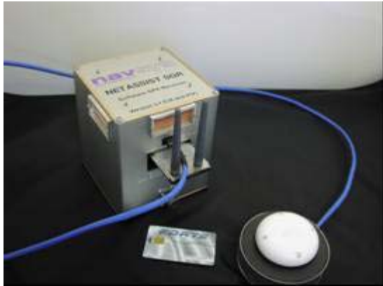
Figure 1: PC/104-Plus SDR Hardware Test bed
