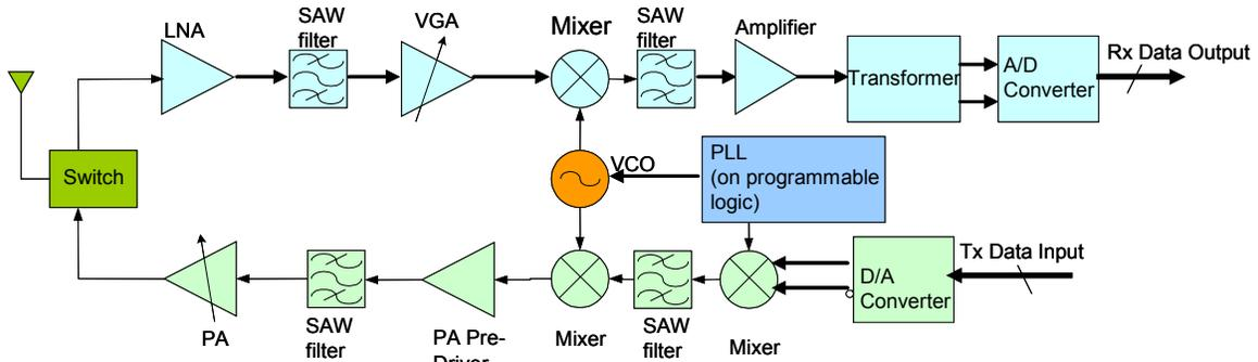
Figure 6: Block Diagram of 900 MHz DAE
