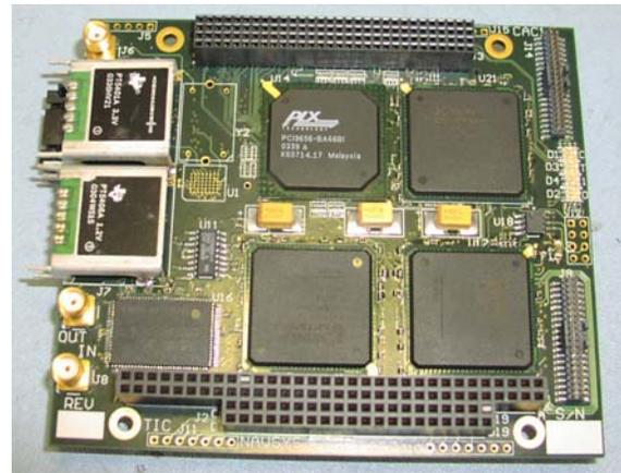
Figure 5: PC/104-Plus FPGA Card
