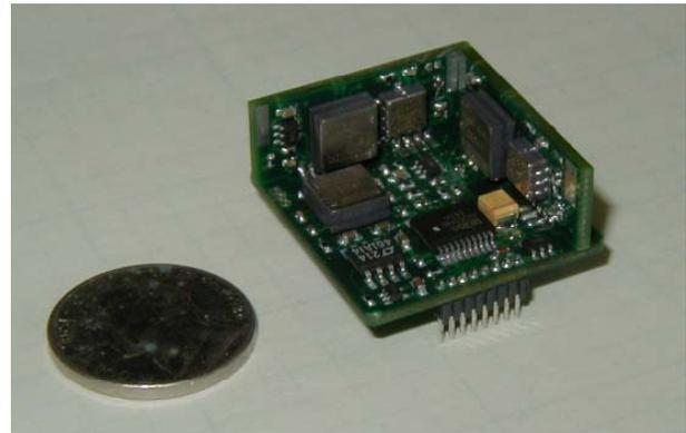
**Figure 7 Small MEMS Inertial Measurement Unit (1"x1"x 0.5")**
