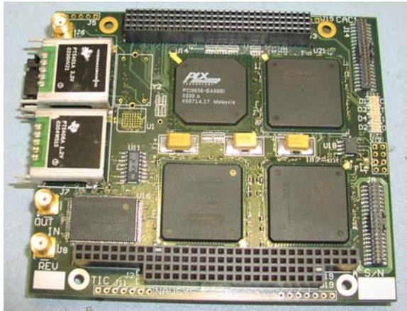
**Figure 6 PC/104-Plus FPGA Card**
