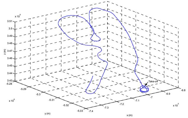
Figure 15 Flight Profile of the F-16 during testing
