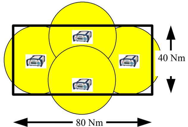
Figure 6 Range Layout (distance between receivers should be ~30 nmi.)
