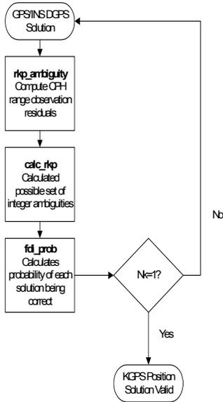
**Figure 10 Kinematic Positioning Algorithm**
