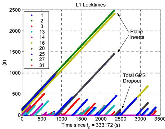
**Figure 19 GPS locktime during the flight**
