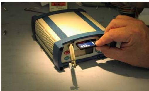
**Figure 8 Data removal from ground system receiver**
