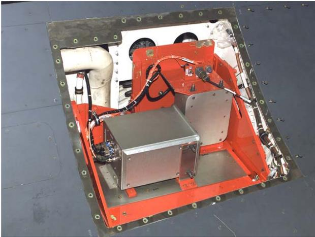
**Figure 1 TSPI Installation in wing root on F-16**
