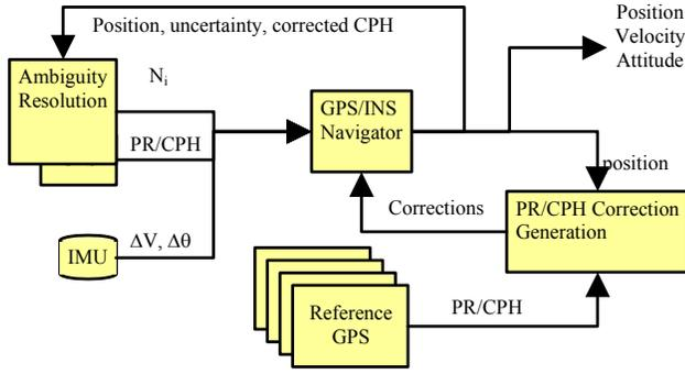
**Figure 9 Kinematic GPS/Inertial Navigation**
