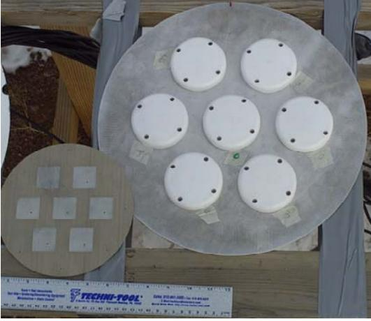
**Figure 3 Seven-Element CRPA and Mini-Array**
