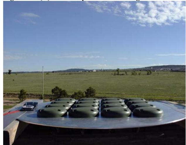
Figure 2 Sixteen Element HAGR Antenna Array
