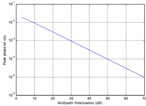
**Figure 16 Multipath Peak Phase error vs. Attenuation (dB)**
