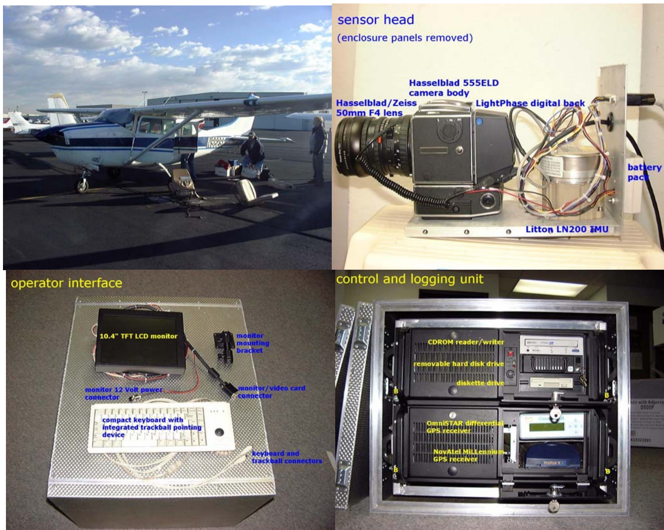
Figure 4 Flight System (clockwise from upper left: aircraft, sensor head with camera and IMU, data logger with display and keyboard, data logger).
