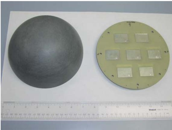
**Figure 1 Seven-inch seven-element dual-frequency (L1/L2) S-CRPA (superstrate hemisphere on the left and substrate on the right)**
