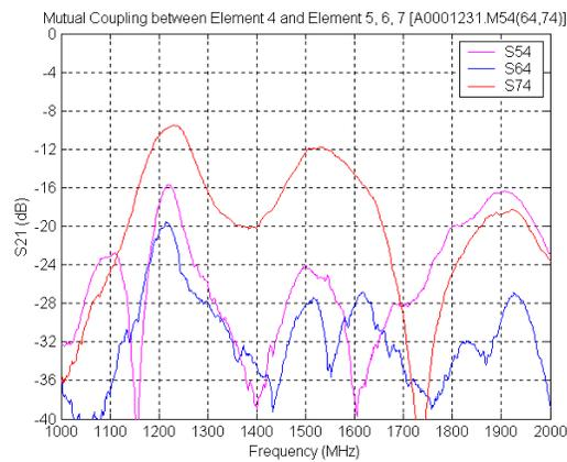
**Figure 21 Mutual coupling between Element 4 and Element 5, 6, and 7**
