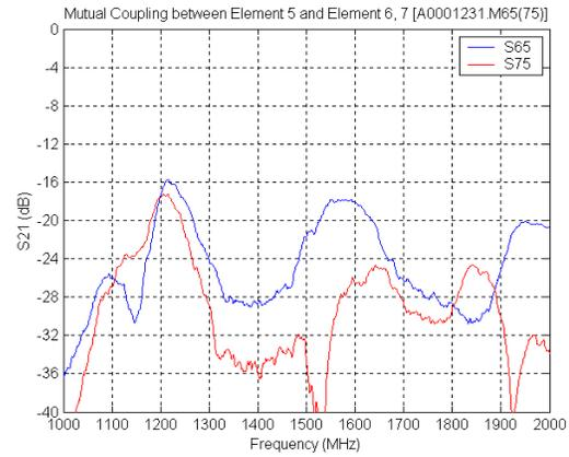
**Figure 22 Mutual coupling between Element 5 and Element 6 and 7**
