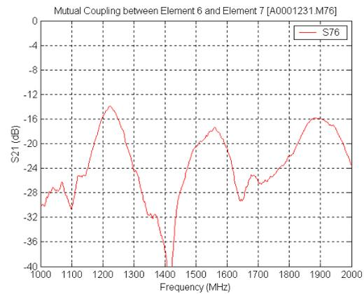
**Figure 23 Mutual coupling between Element 6 and Element 7**
