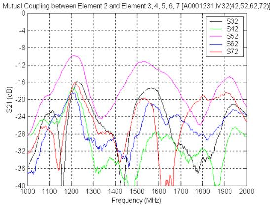
**Figure 19 Mutual coupling between Element 2 and Element 3, 4, 5, 6, and 7**
