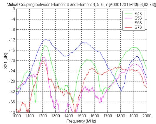
**Figure 20 Mutual coupling between Element 3 and Element 4, 5, 6, and 7**
