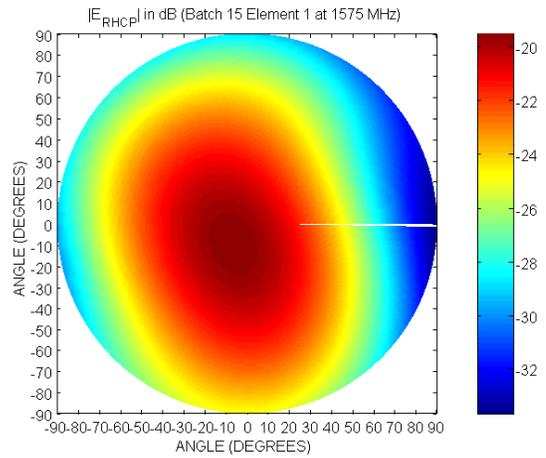
**Figure 8 Simulated RHCP radiation pattern of the center antenna element at 1575 MHz (single probe-feed design)**
