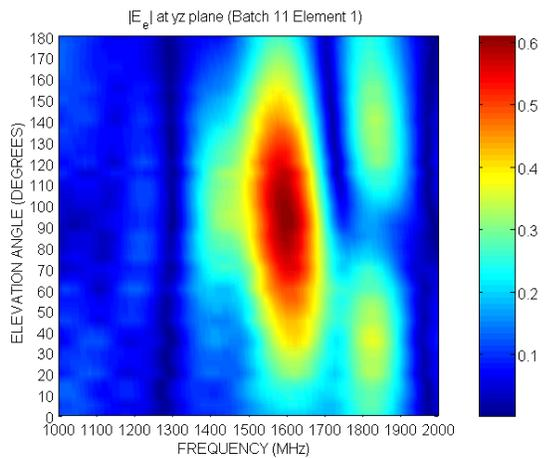
**Figure 7 Simulation of the other orthogonal radiation field components versus elevation angle and frequency (single probe-feed design)**
