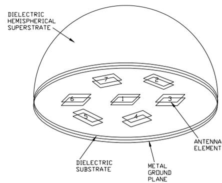
**Figure 1 Configuration of 5.3" 7-element GPS dual-frequency (L1/L2) S-CRPA**
