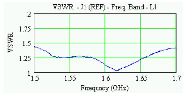
**Figure 11** Measured VSWR of element 1 in L1 band (dual probe-feed design)
