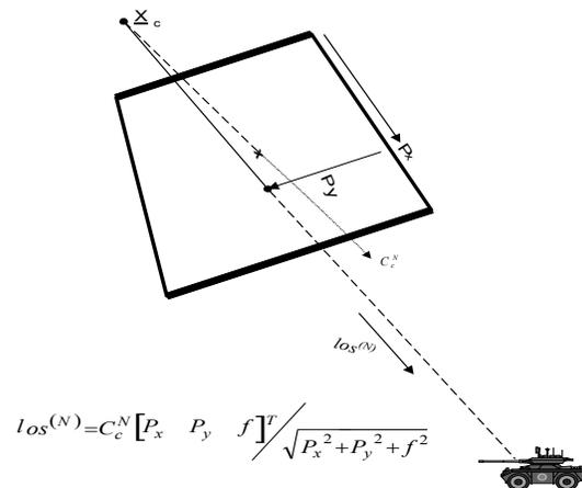
Figure 1 GPS/Inertial Georegistration
