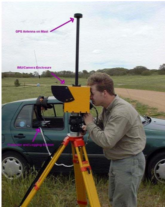
**Figure 8 Terrestrial GI-Eye Hardware**
