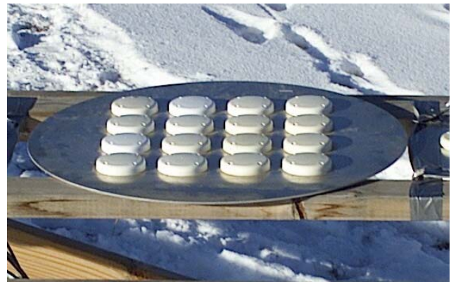
Figure 2 Sixteen Element HAGR Antenna Array
