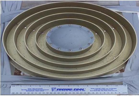
**Figure 9 Choke Ring Antenna (provided by NGS)**
