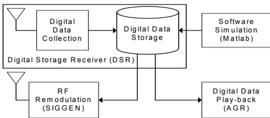
**Figure 1 Advanced GPS Hybrid Simulator Architecture**
