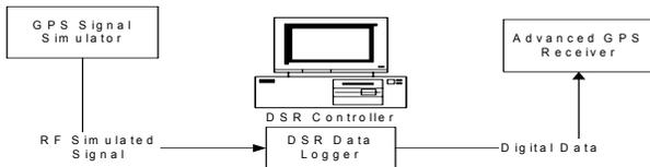
**Figure 11 Digital Storage and Playback Test Set-up**
