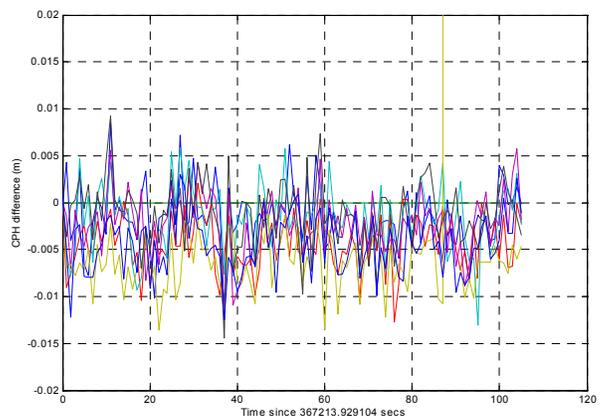
**Figure 8 Double-Differenced Carrier Phase (m)**
