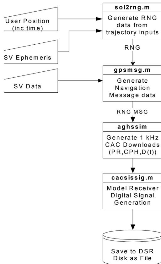
**Figure 5 AGHS MATLAB Signal Simulation**
