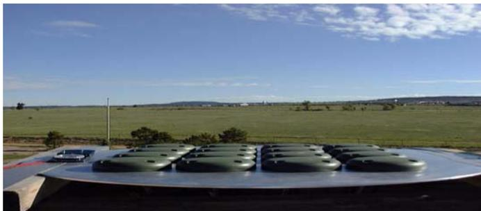
**Figure 2 Sixteen Element L1/L2 Antenna Array**
