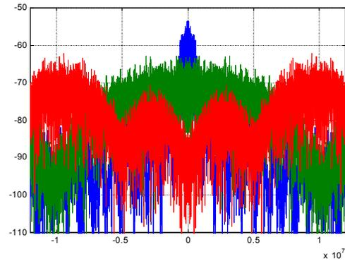
**Figure 4 MATLAB Simulated C/A, P and M-code Signals**
