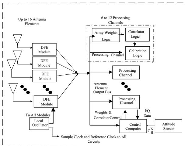
**Figure 6 P(Y) HAGR System Block Diagram**
