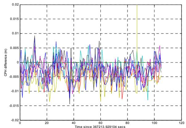
**Figure 8 Double-Differenced Carrier Phase (m)**
