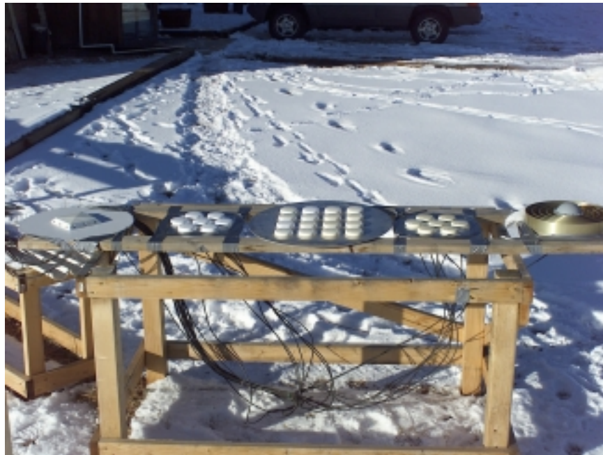
Figure 6 Test Set-up Showing Trimble, HAGR and Ashtech Antennas
