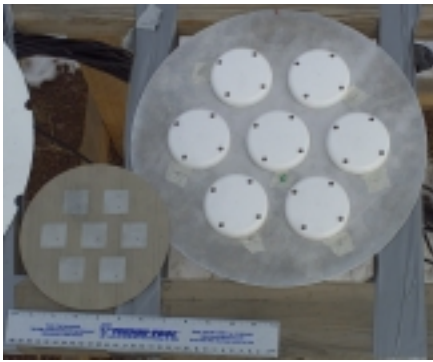
Figure 10 7-Element Antenna and Next Generation Mini-Array
