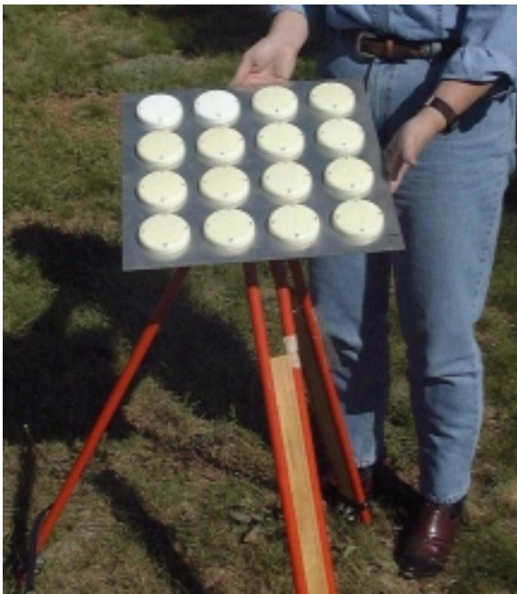
Figure 1 HAGR 16-element antenna array
