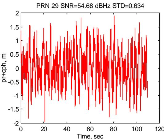
**Figure 7 HAGR Difference between Pseudo-Range and Carrier Phase for PRN 29**
