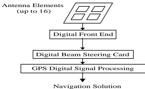
**Figure 2 High Gain Advanced GPS Receiver Design**
